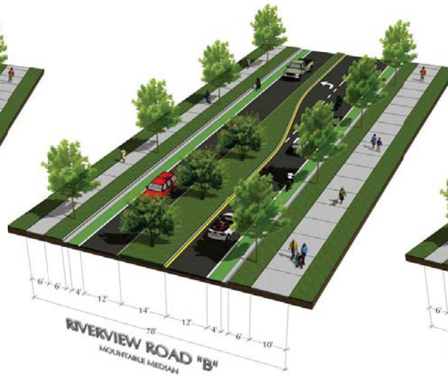
TYPICAL SECTION, INDUSTRIAL STRETCH
