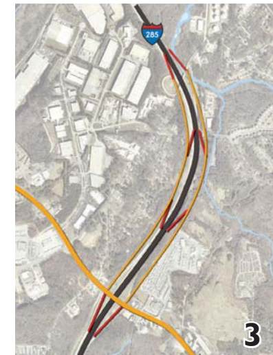
ALT.3: I-285 Collector / Distributor System
