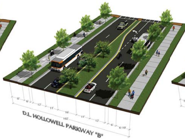
TYPICAL SECTION, INDUSTRIAL STRETCH
