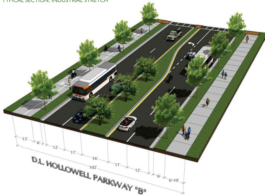
TYPICAL SECTION, INDUSTRIAL STRETCH
