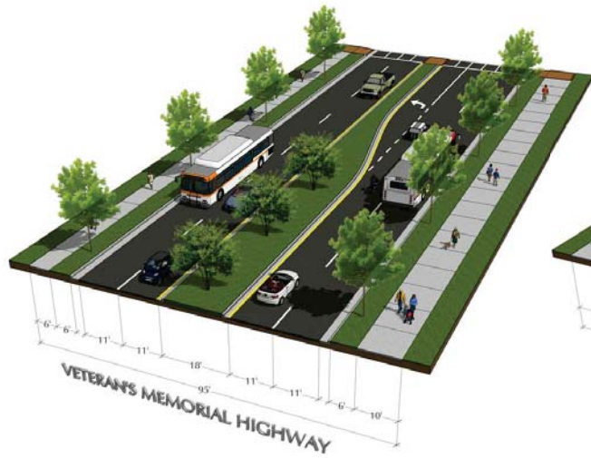
TYPICAL SECTION, SUBURBAN STRETCH
