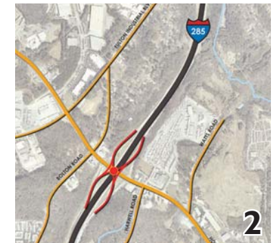
ALT.2: SPUI (Single Point Urban Interchange)
