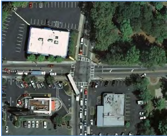
Left: truck attempting to turn from Collier Road onto Howell Mill (Source: Google Earth) Right: pole at same intersection with scrapes due to contact with trucks.
