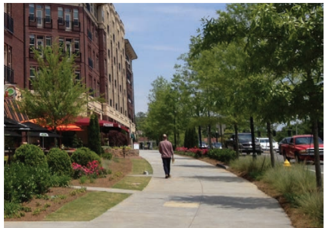
A minimum 7-foot landscape zone between sidewalks and Roswell Road will give pedestrians safety and allow flexibility for sidewalk placement around existing transmission poles.
