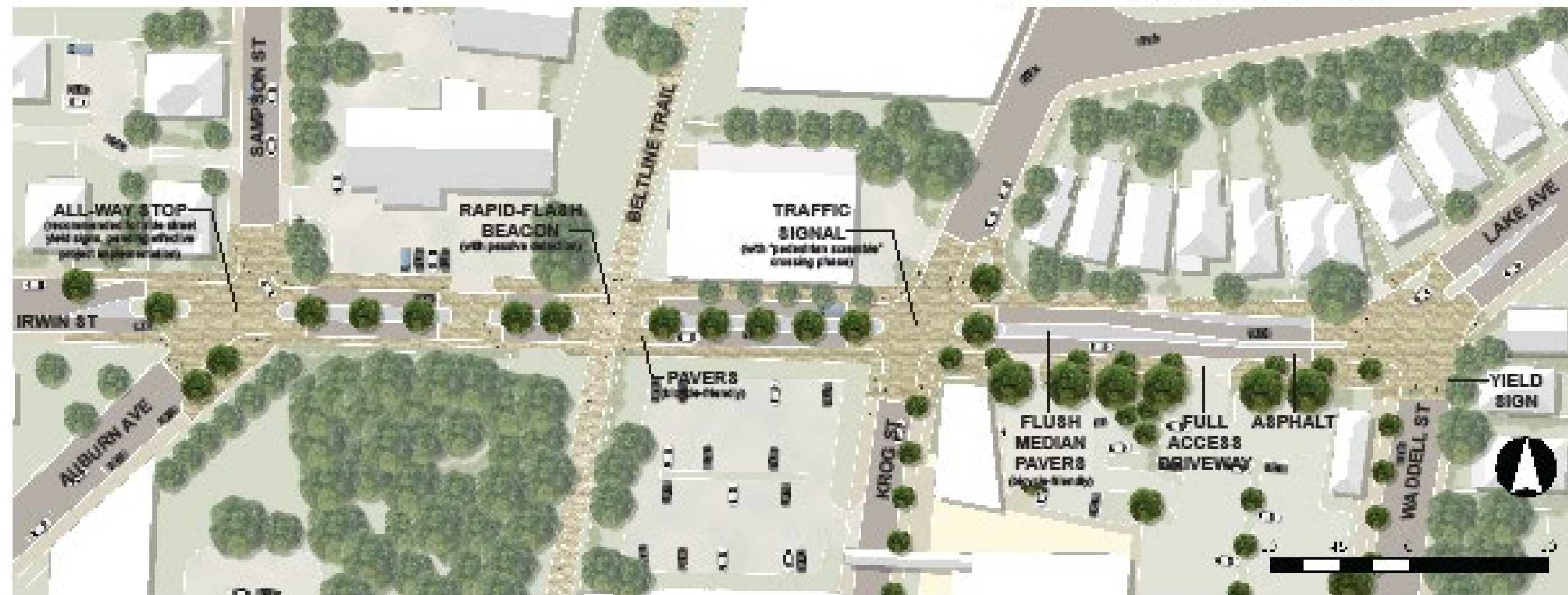
This concept plan shows details of the recommended Irwin Street/Lake Avenue shared space from Sampson Street to Waddell Street
