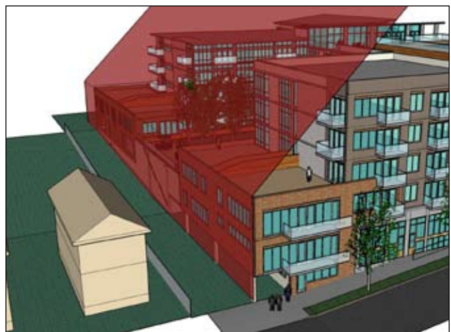
The transitional height plane requires new buildings to step down in height adjacent to existing residential areas
