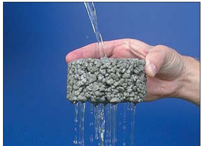
Pervious paving allows water to pass through and infiltrate into the ground
