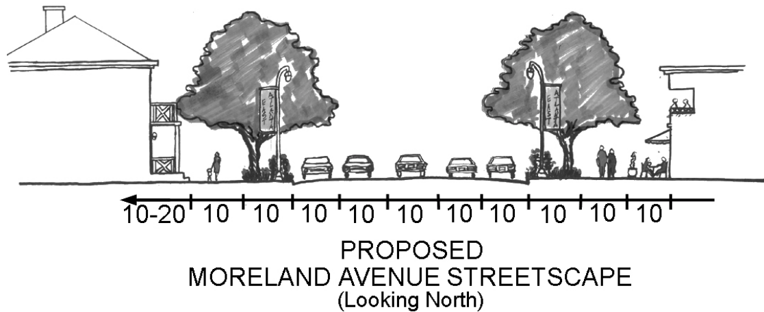
Figure 7: 5 New development on Moreland Avenue will include a ten feet wide landscaped area between the sidewalks and the street, as well as ten feet wide sidewalks and outdoor dining or front yard areas.
