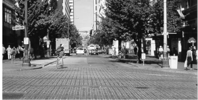
Exposed brick paving serves as a traffic calming device at this intersection in Seattle, Washington.
