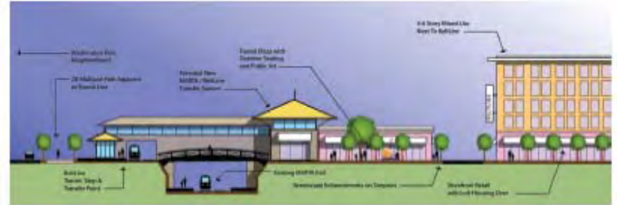
Figure 1. 5 Proposed Beltline Simpson Road Cross Section and New MARTA station
