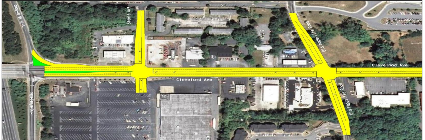
Figure 12. Recommended intersection improvements at Steele Avenue and Old Hapeville Road and road widening on Cleveland Avenue
