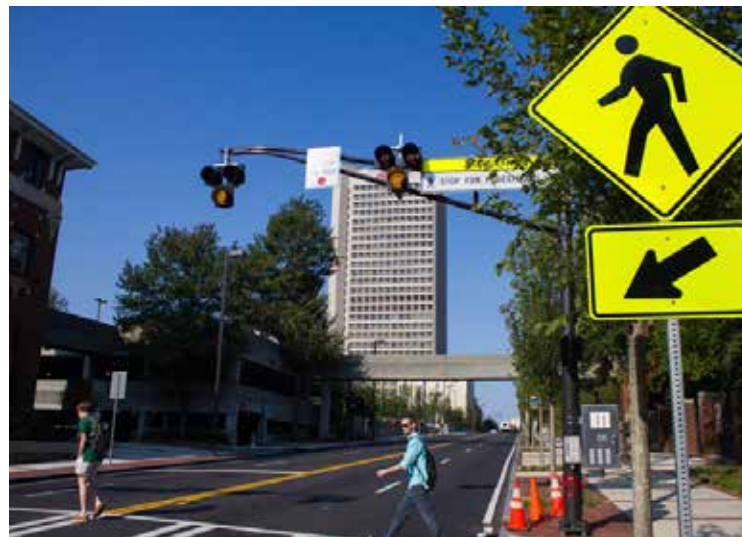
HAWK signal on North Ave on Georgia Tech Campus Image via nique.net
