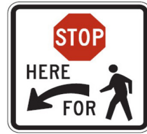
R1-5b signs shall be used for crossings on multi-lane streets.
