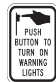
PUSH BUTTON MUTCD R10-24 WITH MODIFIED TEXT FOR RAPID FLASHING BEACON SIZE 9"x15" (affix to push button)
